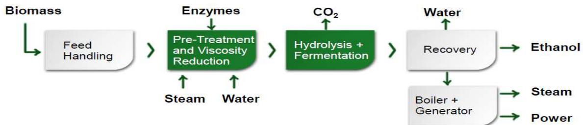
**FIGURE 7. PROCESS FLOW DIAGRAM FOR LIGNOCELLULOSIC ETHANOL PRODUCTION**
